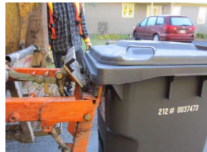
The wheeled bin must be able to hook up to the truck's mechanism
