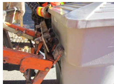
The wheeled bins that cannot be hooked up to the truck's mechanism
